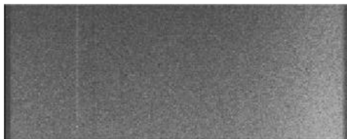
Fig. 5. Low level amplifier glow visible in CCD97
