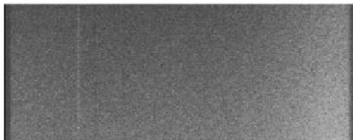
Fig. 5. Low level amplifier glow visible in CCD97
