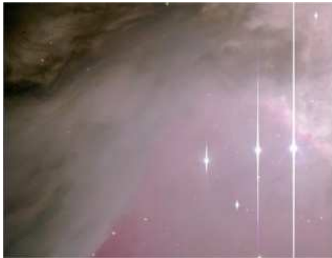
Figure 4: CCD blooming. When a pixel becomes saturated, additional photo-charge will then spill out into neighbouring pixels. Image courtesy of Nik Szymanek.
